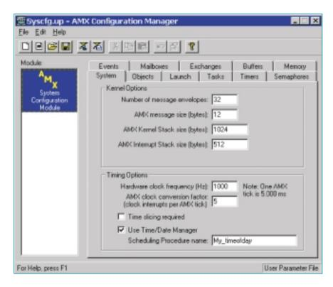
**AMX** is a full featured real time operating system (RTOS) for the ARM and ARM Thumb microprocessor families. AMX has been tested on the Atmel AT91EB40A, EB42, EB63 and AT91SAM7S-EK Evaluation Boards.
